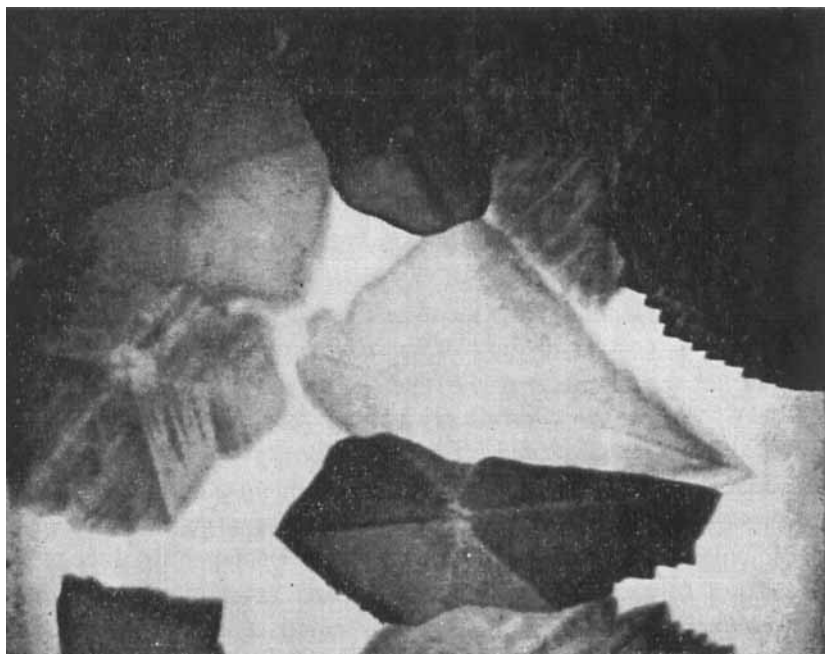
PLATE I. Cyclopentanol freezing at about -18^{\circ}\text{C} showing hexagonal growth patterns. Through crossed polaroids, magnification \times 2 .
